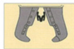
I-beam sheared by shear blades
